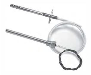
The 310 series thermistor sensors must be wired in series with a 320 series setpoint adjuster. The total resistance is 2200 ohms when the sensor temperature equals the setpoint. The NTC thermistor increases resistance as temperature decreases.
