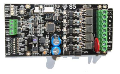
Low cost 24VAC control works with proportional thermostats, building management systems and other digital controls.
