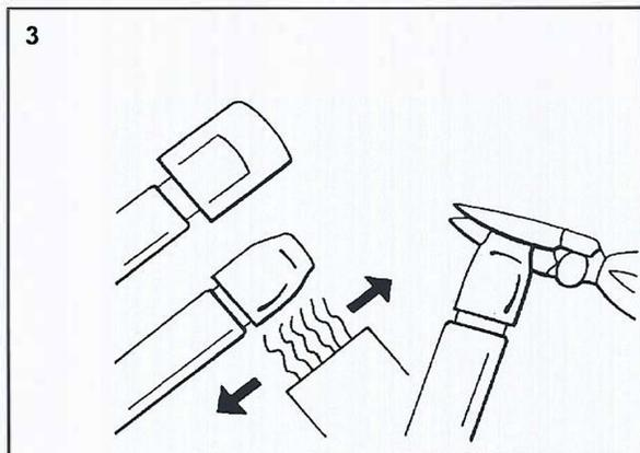
Heat-shrink 1 1/2" heat-shrink tube in place with 3/8" over end of heating cable. Remove heat. Squeeze end with needle-nose pliers. Hold for 10 to 15 seconds.
