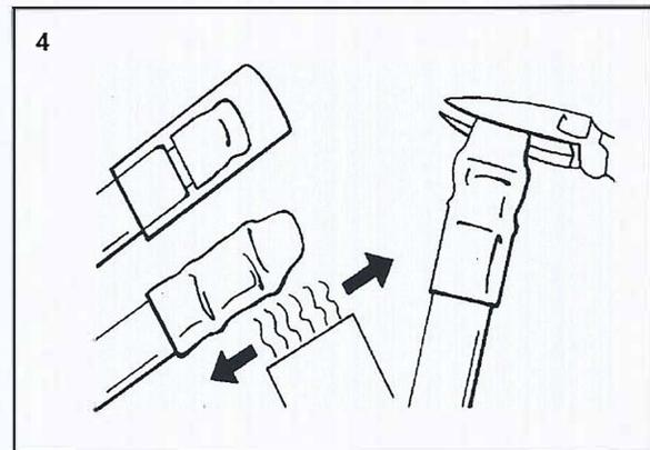
Heat-shrink 4" heat-shrink tube in place with 3/8" over end of smaller heat-shrink tube. Remove heat, resqueeze at end of smaller heat-shrink tube, then squeeze at end of outer heat-shrink tube. Hold for 10 to 15 seconds.
