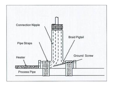
Connect the lead wires to the screws on the 5. light fixture. Fill the connection nipple with the silicone sealant. Stow any excess lead wire in the box and mount the light fixture into the box. Attach the box cover to the box and attach the caution label to the cover.
