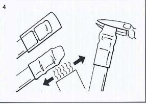
Heat-shrink 4" heat-shrink tube in place with <sup>3</sup>/<sub>6</sub>" over end of smaller heat-shrink tube. Remove heat, resqueeze at end of smaller heat-shrink tube, then squeeze at end of outer heat-shrink tube. Hold for 10 to 15 seconds.
