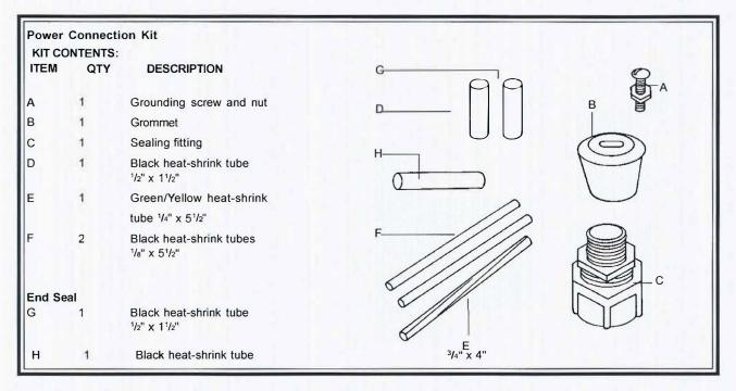
WARNING - The contents of the component kit must be installed correctly to ensure proper operation and to prevent shock or fire. Read these important warnings and carefully follow all the installation instructions.
