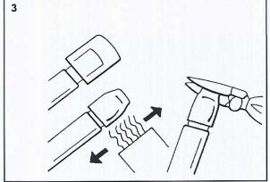
Heat-shrink  $1'h^{a}$  heat-shrink tube in place with  $36^{a}$  over end of heating cable. Remove heat. Squeeze end with needle-nose pliers. Hold for 10 to 15 seconds.
