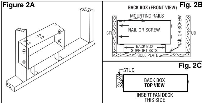
1. Locate back box and back box support brackets (2). Back box must be installed with mounting rails to the top (see Figure 2B)
